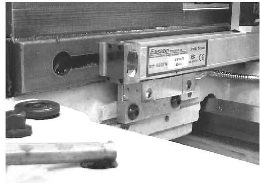
Testing for parallel can be done by either a dial indicator or a precision level
